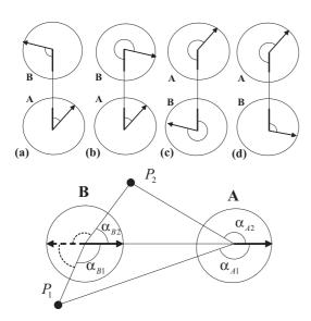
Fig. 2. Four possible 2D reconstructions from the epipoles between two views extracted from the 1D trifocal tensor (top). The relations between the angles of the projections of matched points (e.g.  $P_1$  and  $P_2$ ) in two aligned views can be used to resolve the 2D reconstruction ambiguities (below).
