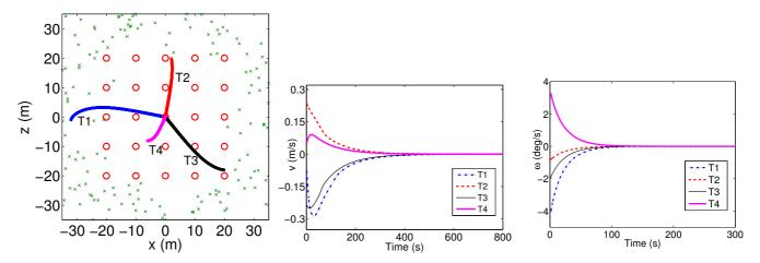
Fig. 6. Simulation results. Left: robot paths for four different trajectories with a reference set consisting of 25 images acquired in positions forming a grid. The goal view is at position (0,0) for all the trajectories. The locations of the reference images are marked as circles. The cloud of 200 points used to compute the 1D trifocal tensors is also shown. Center: Linear velocity for the four trajectories. Right: angular velocity for the four trajectories.
