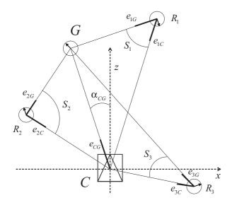
Fig. 5. Elements involved and angles employed in the homing strategy. C is the robot's current location, at the coordinate origin. G is the goal location.  $R_i$  are reference views. Three of the n views on the reference set are depicted as example.
