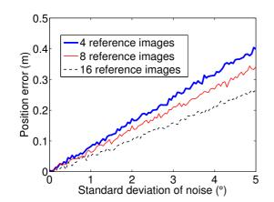
Fig. 8. Simulation results: final position error as a function of added Gaussian noise for reference sets of 4, 8 and 16 images.
