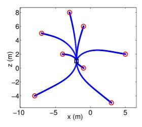
Fig. 7. Simulation results: robot paths with 8 reference images in arbitrary locations. The different paths obtained by taking each of the reference images (marked as circles) as the goal, from a common starting location (marked as a square), are shown.
