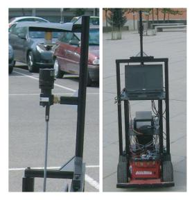
Fig. 9. Omnidirectional camera (left) and complete setup (right) used for the first indoor experiment and the outdoor experiment.
