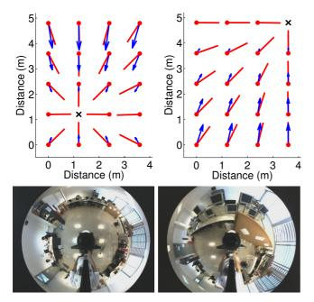
Fig. 10. Top: displacement vectors (arrows) and directions of the epipoles (line segments) with respect to the goal estimated at every reference position for two different goal locations (marked with a cross) in the real setting of the first indoor experiment. Bottom: goal images corresponding to the homing vector representations on top.
