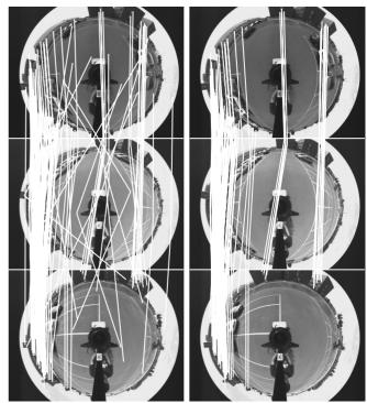
Fig. 14. Example of a trio of images from the outdoor data set with their putative SIFT correspondences joined by lines (left). Feature matches remaining after the robust computation of the 1D trifocal tensor (right).
