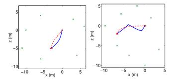
Fig. 17. Homing paths from two different initial locations to the goal location situated in (0,0), with seven (left) and eight (right) feature matches. The paths generated by the method proposed by Argyros et al. [10] (solid line) and the paths generated by the approach presented in this paper (dashed line) are shown.
